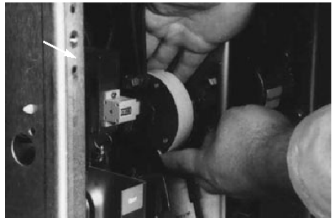
Figure 6-8 Attaching Tape Around to Back of Cam
